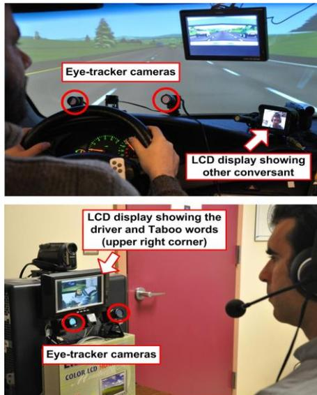
Figure 1: a) Driver and b) remote conversant.
