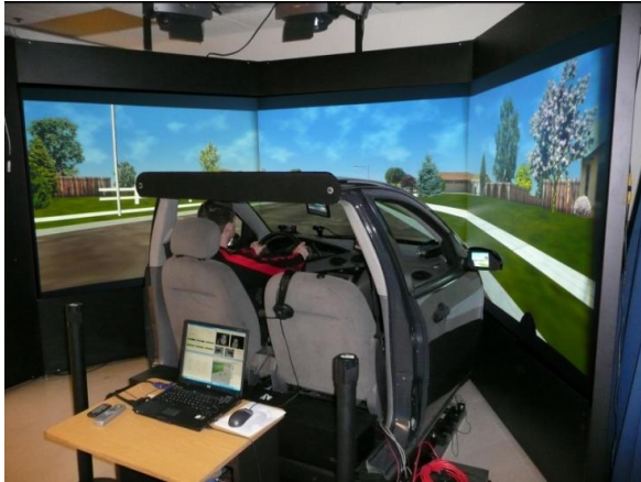
Figure 1. 180° field of view driving simulator.
